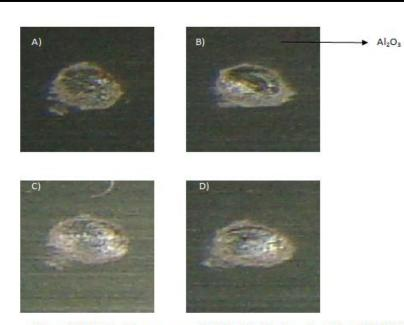
Figure (A3) Optical Images magnified (1x20) after Irradiated by Nd-YAG Pulsed laser A) 24 volts B) 21 volts C) 19 volts D)15.5 volts (Surface Treated by laser Before Anodizing) Anodizing Time is 30 Minutes, 360mJ energy, 3x10-9 pulsed duration
