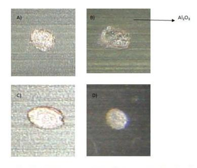
Fig (A4) Optical Images magnified (1x20) after Irradiated by Nd-YAG Pulsed Laser A) 24 volts B) 21 volts C) 19 volts D)15.5 volts (Surface was not Treated by Laser Before Anodizing) Anodizing Time is 30 Minutes, 360mJ energy, 3x10-9 pulsed duration
