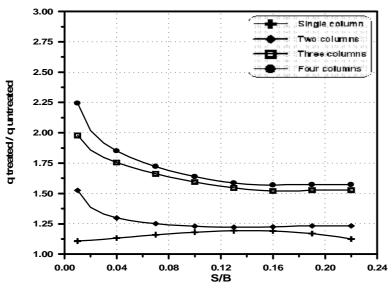
Figure (12) Bearing improvement ratio versus (S/B) for the soil treated with stone columns, cu = 12 kPa and L/D = 6.
