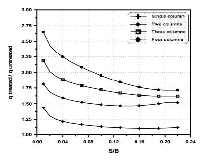
Figure (18) Bearing improvement ratio versus (S/B) for the soil treated with stone columns, cu = 12 kPa and L/D = 8.
