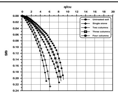
Figure (17) q/cu versus S/B for the soil treated with stone column cu = 12 kPa an L/D = 8.
