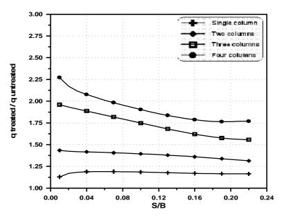
Figure (10) Bearing improvement ratio versus (S/B) for the soil treated with stone columns, cu = 9 kPa and L/D = 6.
