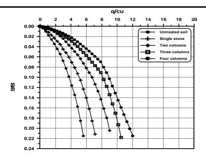
Figure (15) q/cu versus S/B for soil treated with stone column cu = 9 kPa and L/D = 8.
