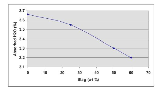
Figure (2) The Relation Between Slag Content and Absorbed Water (%) by Weight .
