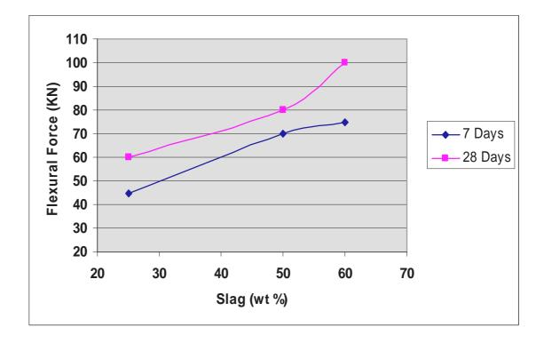
Figure (4) The Effect of Slag Content on the Flexural Strength Property for Cylindrical Samples After 7 and 28 Days
