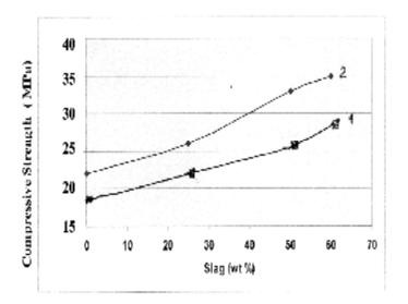
Figure (3) The Relation Between Compressive Strength After 7 and 28 Days and Slag Content 1- After 7 days 2-After 28 days
