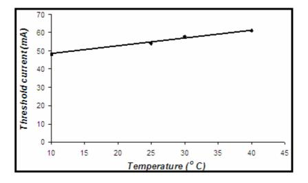
Fig (7) The threshold current as a function of the temperature
