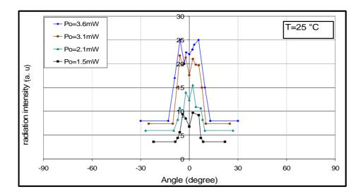
Fig (10) Power dependence of far pattern (parallel junction)
