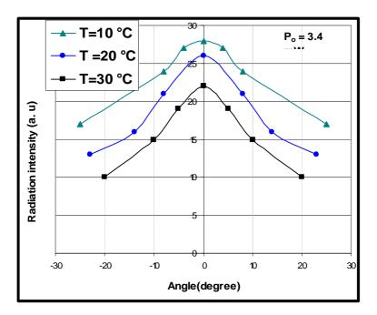
Fig (11) Temperature dependence of far pattern (perpendicular to junction)
