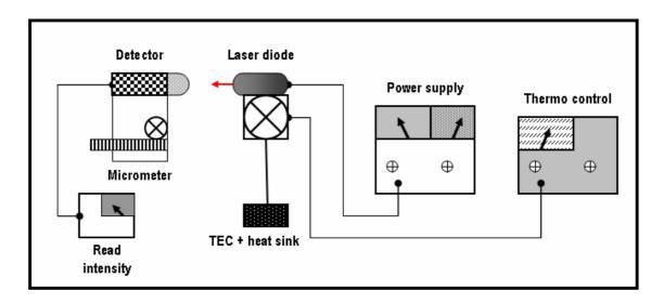
Fig (4) The Measured beam divergence angle.
