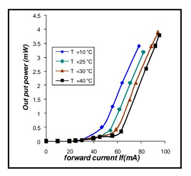
Fig(6) Output power of the laser diode as a function of the injection current at different temperature.
