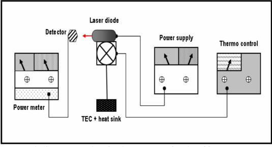
Fig (3) The Measuring of optical power as a function of forward current.
