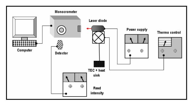
Fig (5) Measured the emission spectrum for laser diode
