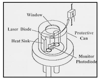
Fig (2) structure of laser diode.
