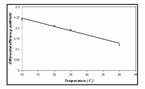
Fig (8) Differential Efficiency & Temperature Characteristics
