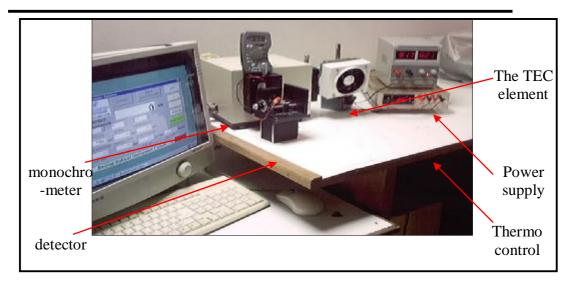
Fig (1)A photograph of the layout on the optical table
