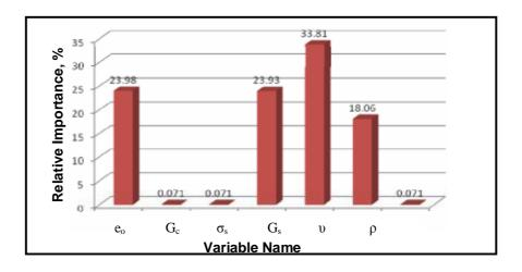
Fig. (1) Relative importance of the input variables for model (S/B)<sub>w</sub>.
