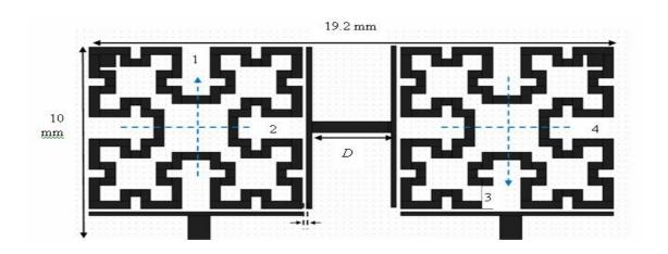
Figure (8) The layout of the modeled four pole 2<sup>nd</sup> iteration MLPF microstrip resonator filter at a frequency of 2.4 GHz
