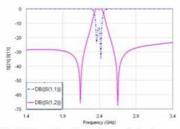
Fig(10) Return loss, S<sub>11</sub>, and transmission, S<sub>21</sub>, responses of a two pole conventional square ring microstrip resonator filter
