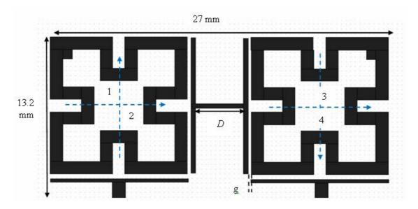
Figure (7) The layout of the modeled four pole  $\mathbf{1}^{st}$  iteration MLPF microstrip resonator filter at a frequency of  $\mathbf{2.4~GHz}$
