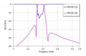
Fig(14) Return loss, S<sub>11</sub>, and transmission, S<sub>21</sub>, responses of four pole double square ring microstrip resonator filter
