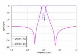
Fig(11) Return loss, S<sub>11</sub>, and transmission, S<sub>21</sub>, responses of a two pole 1st iteration MLPF microstrip resonator filter
