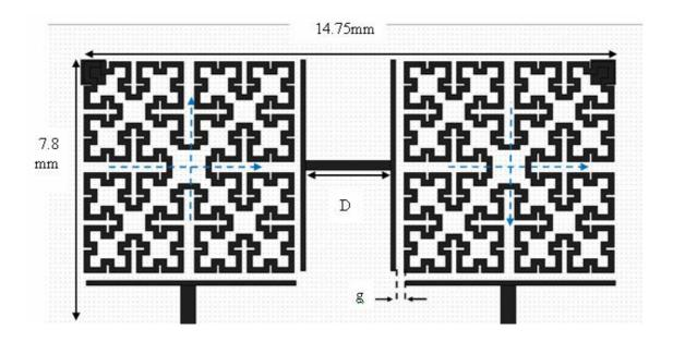
Figure (9) The layout of the modeled four pole  $3^{rd}$  iteration MLPF microstrip resonator filter at a frequency of 2.4 GHz
