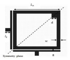
Fig.(2) The layout of the modeled dual- mode 2<sup>nd</sup> iteration MLPF microstrip resonator filter
