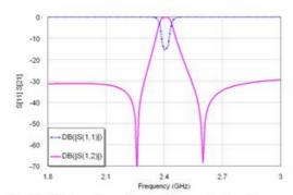
Fig(12) Return loss, S<sub>11</sub>, and transmission, S<sub>21</sub>, responses of the two pole 2<sup>nd</sup> iteration MLPF microstrip resonator filter
