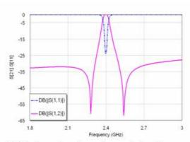
Fig(13) Return loss, S<sub>11</sub>, and transmission, S<sub>21</sub>, responses of the two pole 3<sup>rd</sup> iteration MLPF microstrip resonator filter
