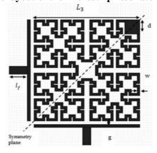
Figure(5) The Layout of the modeled  $3^{\rm rd}$  iteration MLPF microst1rip resonator filter
