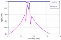
Fig(15) Return loss,  $S_{11}$ , and Transmission,  $S_{21}$ , responses of four pole 1st iteration MLPF microstrip resonator filter
