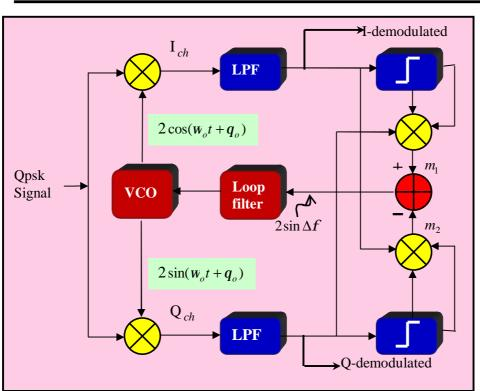
Figure (4) Costas loop for QPSK synchronizer
