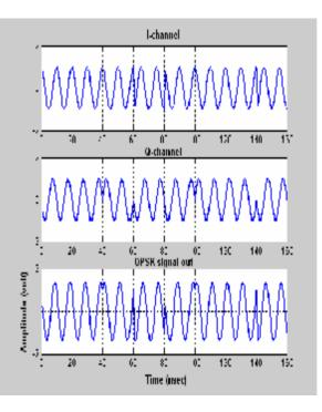
Figure (19) Simulation results of the transmitter of QPSK system
