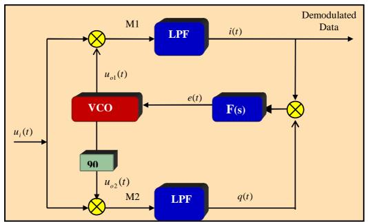
Figure (3) The conventional Costas loop for BPSK
