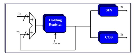
Figure (5) Direct digital frequency synthesizer (DDS)
