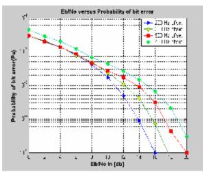
Figure (10): Simulation results of the BPSK signal for frequency offset from 200 to 700 Hz offsets
