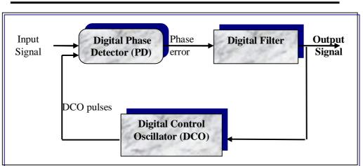
Figure (2): Block diagram of digital phase locked loop
