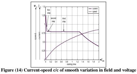
$(t_1 = 0.057, t_2 = 0.18 \text{ and } t_3 = 1.04)$
