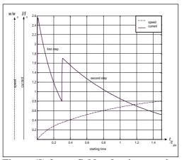
Figure (8) 2 step field reduction starting
