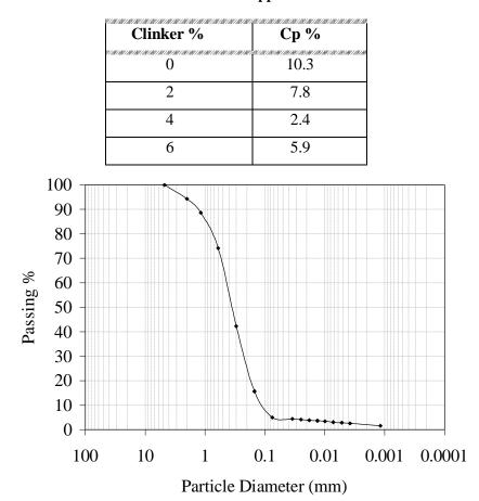
Table (3) Results of double oedometer test for treated soil at 200 kPa applied stress
