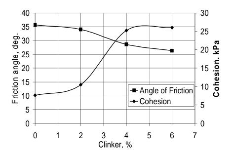
Figure (9) Variation of shear strength parameters with clinker material.
