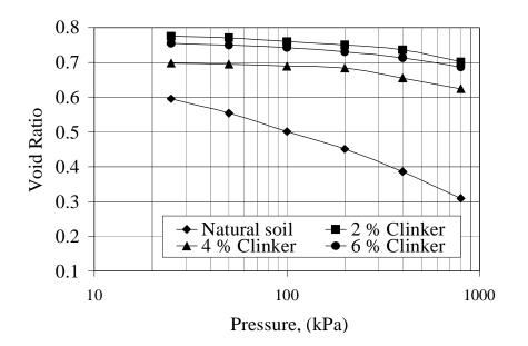
Figure (6) Applied stress vs. void ratio at soaking state.
