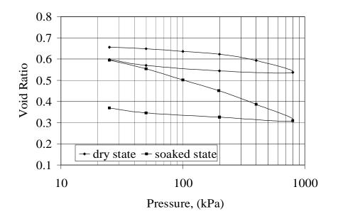
Figure (3) Results of double oedometer test for the natural soil.
