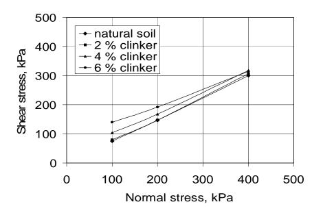
Figure (8) Results of direct shear tests.
