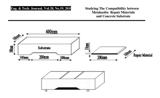
Figure (5) Third point loading composite beam
