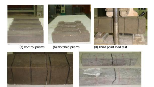
(e) Substrate failure (f) Repair material failure Figure (6) Compatibility test samples for composite beam of the research
