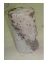
(c) Repair material failure
