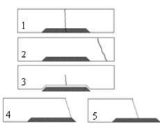
Figure (4) Probable failures of the composite beam; 1,2 – compatible; 3, 4 and 5- incompatible [14]
