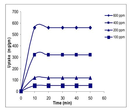
Figure (7) Effect of contact time on phenol uptake by 0.75 gm WT-GAC
