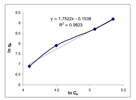
Figure (14) plot of (lnq<sub>e</sub>) vs (lnC<sub>e</sub>) for determination of Freundlich constant at 4gm WT
