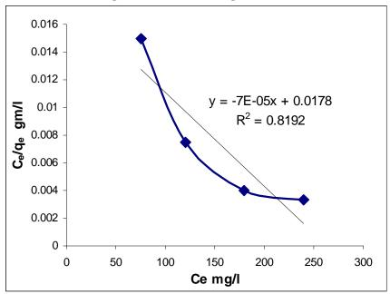
Figure (19) plot of (C<sub>e</sub>/q<sub>e</sub>) vs (C<sub>e</sub>) for determination of Langmuir constant at 0.5gm WT-GAC
