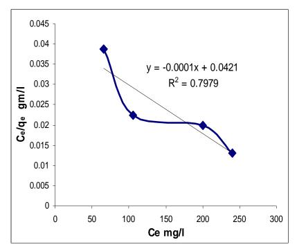
Figure (12) plot of (C<sub>e</sub>/q<sub>e</sub>) vs (C<sub>e</sub>) for determination of Langmuir constant at 2gm WT
