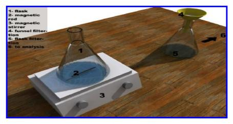
Figure (1) Batch adsorber apparatus
