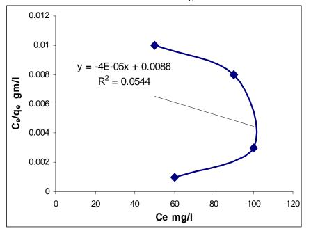
Figure (17) plot of (C<sub>e</sub>/q<sub>e</sub>) vs (C<sub>e</sub>) for determination of Langmuir constant at 1gm WT-GAC
