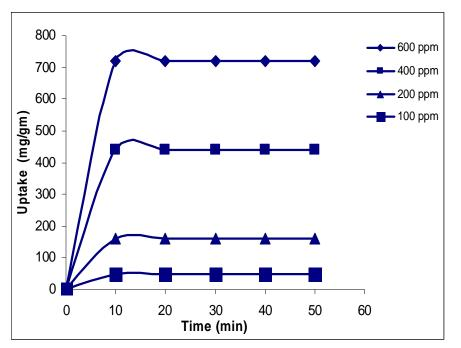
Figure (8) Effect of contact time on phenol uptake by 0.5 gm WT-GAC
