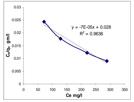
Figure (13) plot of (C<sub>e</sub>/q<sub>e</sub>) vs (C<sub>e</sub>) for determination of Langmuir constant at 1gm WT
