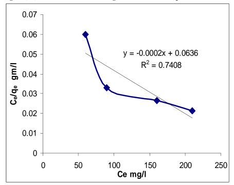
Figure (11) plot of (C<sub>e</sub>/q<sub>e</sub>) vs (C<sub>e</sub>) for determination of Langmuir constant at 4gm WT
