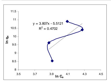
Figure (20) plot of (lnq<sub>e</sub>) vs (lnC<sub>e</sub>) for determination of Freundlich constant at 1gm WT-GAC
