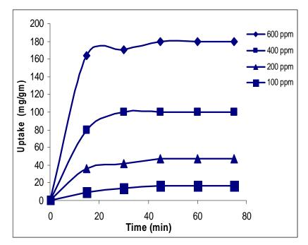
Figure (4) Effect of contact time on phenol uptake by 2 gm WT
