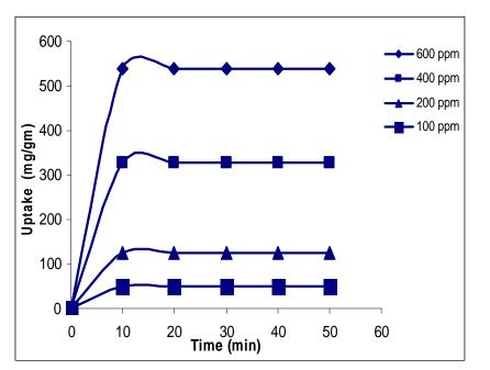
Figure (6) Effect of contact time on phenol uptake by 1 gm WT-GAC
