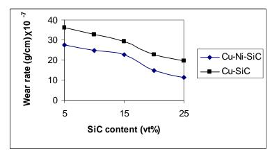
Figure (5) Variation of wear rate with Sic content for (5N) loaded
