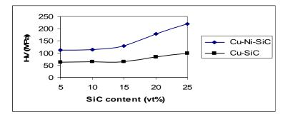
Figure (3) Variation of Vickers micro hardness with Sic content
