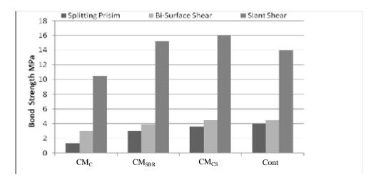
Figure (4) Effect of different bond tests and different types of repair materials on the bond strengths value
