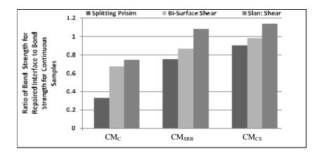
Figure (5) Effect of type of repair material and bond test on the ratio of bond strength of repaired interfaces to that for continuous specimens
