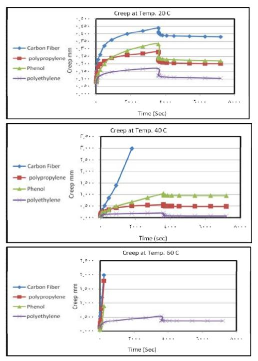
Figure (6) Creep Test at different Temperature 6426
