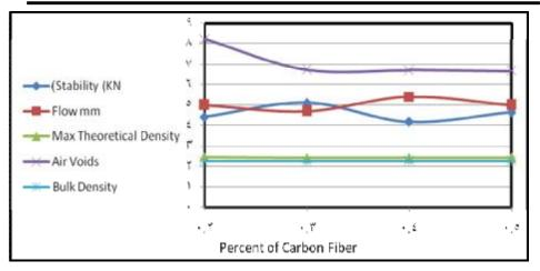
Figure (4) Marshall Properties of Stone Matrix Asphalt.
