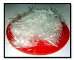
**B**, **Polypropylene** Fiber Figure (2) Fibers used in this Study
