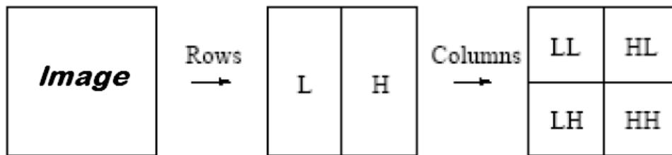
Figure (2): One DWT decomposition step [9]
