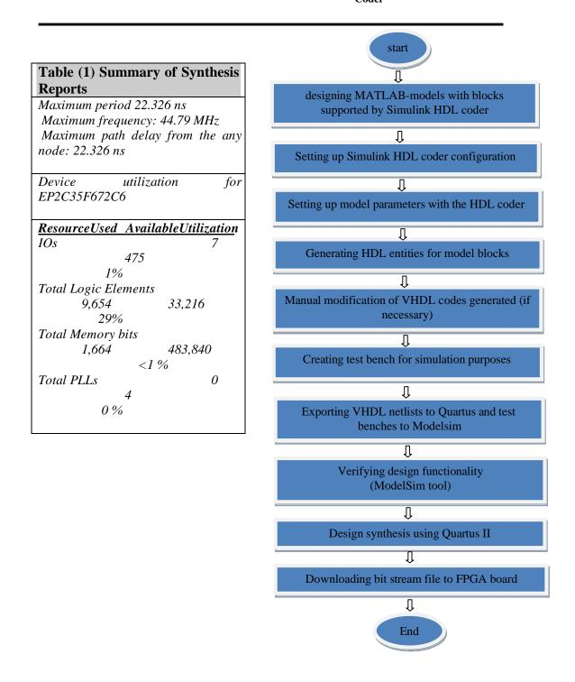
Figure (1) Design flow for realizing MATLAB-Simulink models using FPG A Boards
