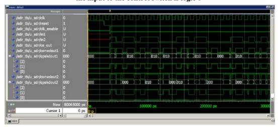
Figure (9) the convolution encoder and QPSK demodulator outputs
