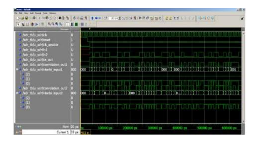
Figure (13) the convolution encoder outputs and viterbi decoder inputs
