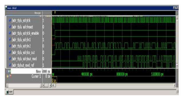
Figure (7) the input and output waveforms when the input to control switch is logic 1
