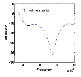
Figure.5. Simulated S<sub>11</sub>Parameter of antenna with MTM
