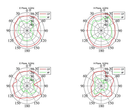
Figure.9 Radiation pattern of the antennas in 4GHz and 9GHz
