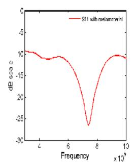
Figure.6. Measured S<sub>11</sub> parameter of the antenna
