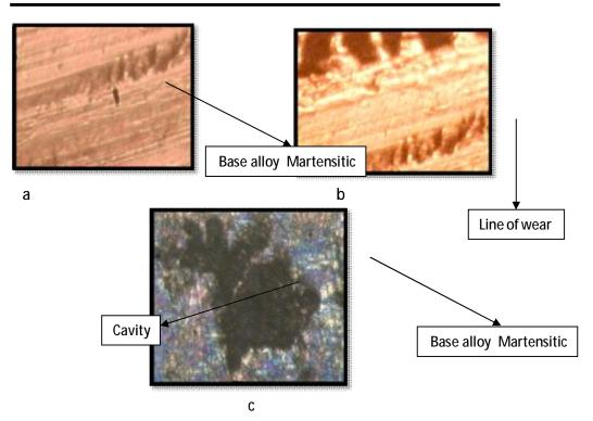
Figure (10)a- Surface of alloy after Quenching in iced water (750X). b-Surface of alloy in quenching case after dry sliding wear (750X).
