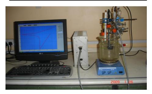
Figure (1) Potentio static equipment
