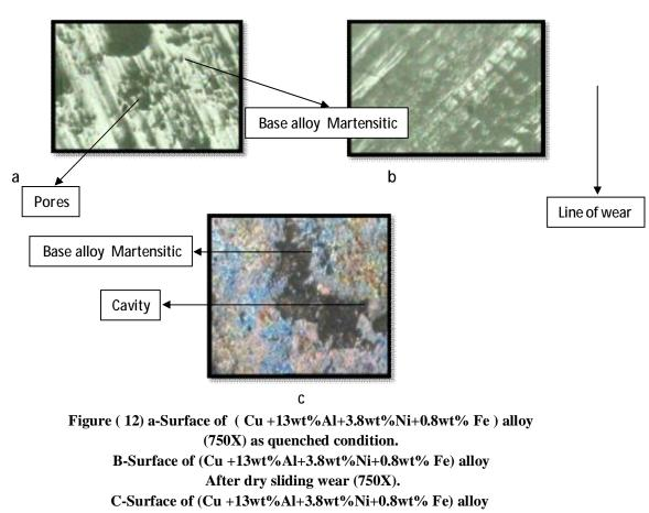
After corrosion test (750X).
