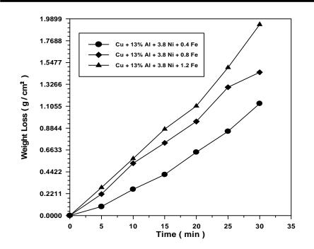
Figure (3) Shows the relation between weight loss during dry sliding with time for (Cu + 13wt%Al + 3.8wt%Ni) alloy with the effect of Fe additives
