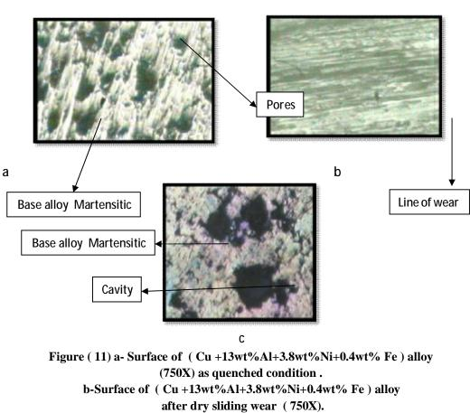
c-Surface of (Cu +13wt%Al+3.8wt%Ni+0.4wt% Fe) alloy after corrosion test (750X).
