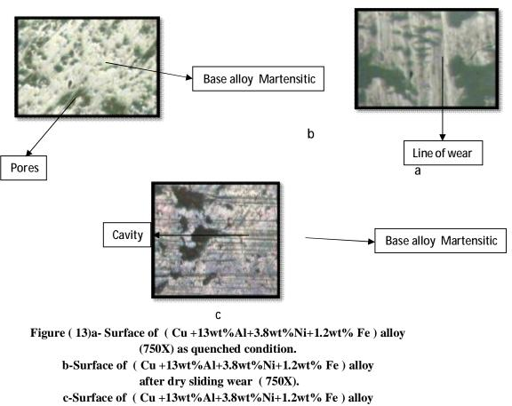
after corrosion test (750X).
