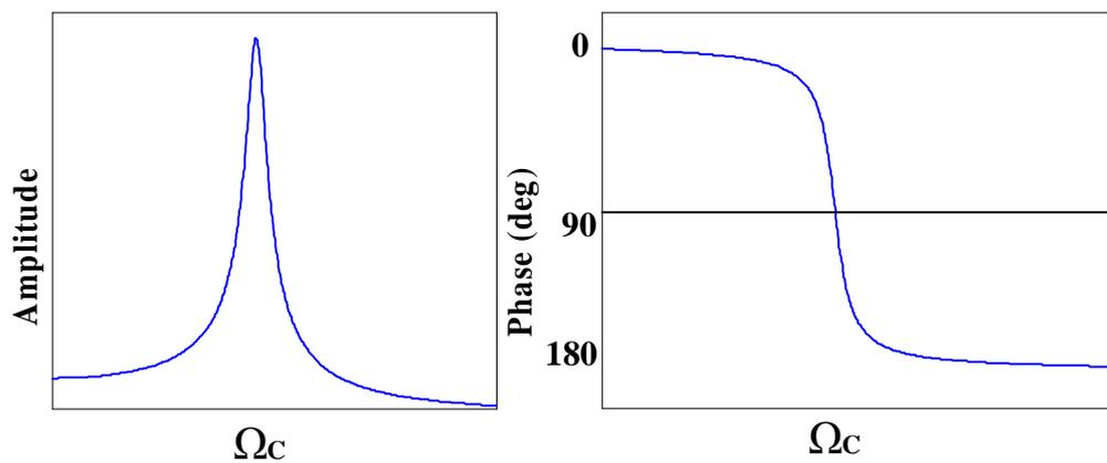
Fig.(2) Synchronous Response Diagram.
