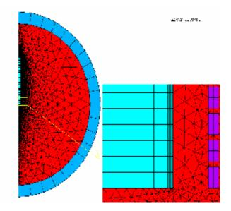
Figure (4) Meshed model of induction heating furnace
