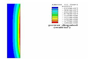
Figure (9) Distribution of the power dissipated per unit volume inside the workpiece
