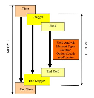
Figure (5) The algorithm of multifield solver
