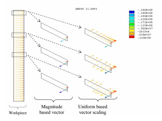
Figure (8) Eddy current density inside the workpiece
