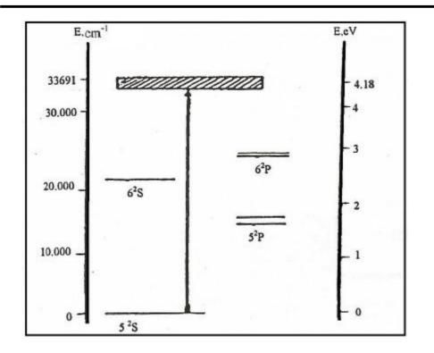
Figure (1) Energy level Scheme for Rb Atom<sup>[8]</sup>
