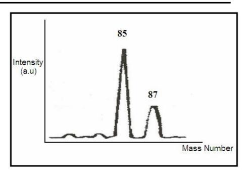
Figure (4) Rubidium isotopes (Rb<sup>85</sup>,Rb<sup>87</sup>) at T= 850 °C using quadruple ion source (I=20 x 10<sup>-11</sup> Amp.)
