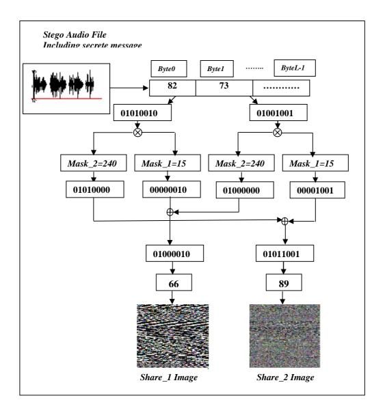
Figure (4): Example of Splitting Stego cover into 2-share two random images
