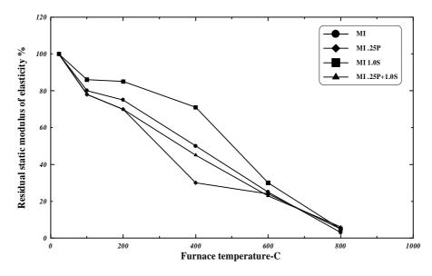
Fig.(3) Effect of polypropylene, steel and hybrid fibers on static modulus of elasticity of LWAC exposed to elevated temperatures
