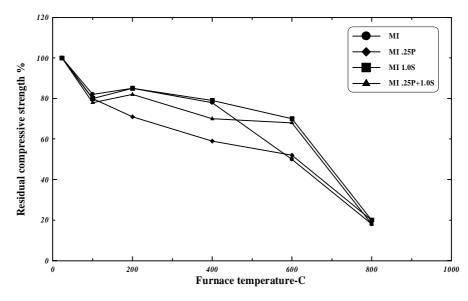
Fig.(1) Effect of polypropylene, steel and hybrid fibers on compressive strength of LWAC exposed to elevated temperatures
