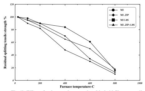
Fig.(2) Effect of polypropylene, steel and hybrid fibers on splitting tensile strength of LWAC exposed to elevated temperatures
