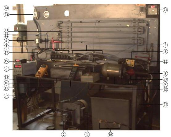
Figure (3) The Test Bench of Hydraulic System
