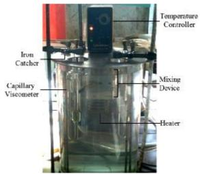
Figure (4) The Viscosity Measuring Device
