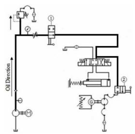
Figure (5) The Schematic Diagram of the Neutral Circuit
