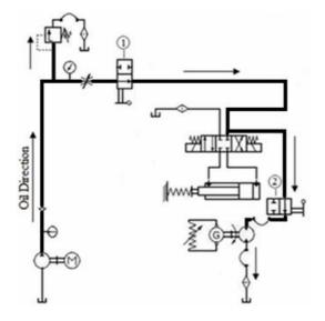
Figure (6) The Schematic Diagram of the Loading Circuit
