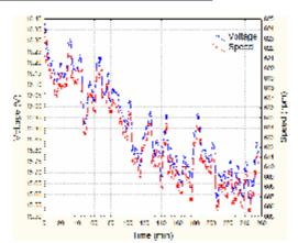
Figure (24) Voltage and Speed Variation with Time at 30 bar
