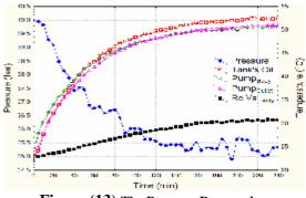
Figure (13) The Pressure Drop and Temperatures Raising With Time (Loading Case)
