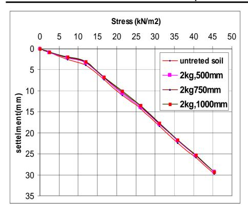
Figure (7) Stress-settlement curve for untreated and treated soil using dynamic compaction(weight 2kg, heights of drop 500,750,1000mm).
