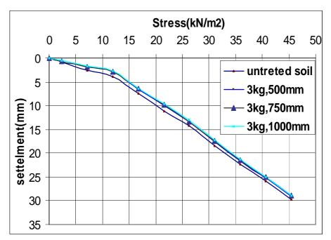
Figure (8) Stress-settlement curve for untreated and treated soils using dynamic compaction (weight 3kg, heights of drop 500,750,1000mm).
