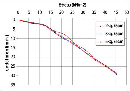
Figure (11) Stress-settlement curve for untreated and treated soils using dynamic compaction (weights 2,3, 5kg heights of drop 750mm).
