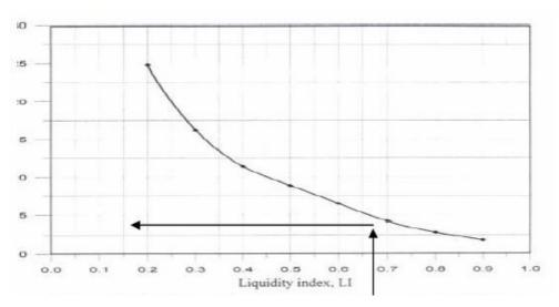
Figure (4) . Variation of undrained shear strength versus liquidity index forremolded clay after 48 hrs.
