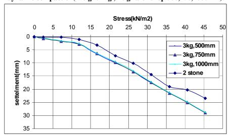
Figure (15) Stress-settlement curve for treated soil using 2 stone columns and dynamic compaction (weight 3kg, heights of drop 500,750,1000mm).
