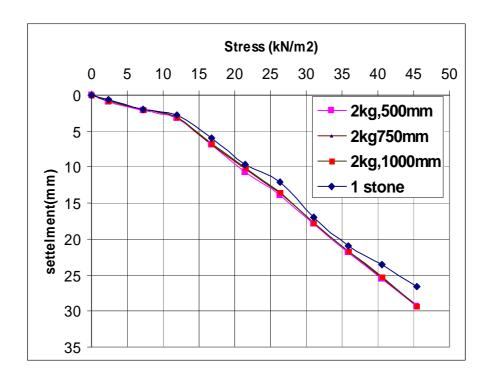
Figure (14) Stress - settlement curve for treated soil using 1stone column and dynamic compaction (weight 2kg, heights of drop 500,750,1000mm).
