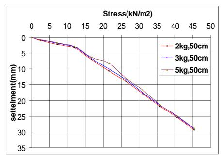
Figure (10) Stress-settlement curve for untreated and treated soils using dynamic compaction (weight2,3, 5kg heights of drop 500mm).
