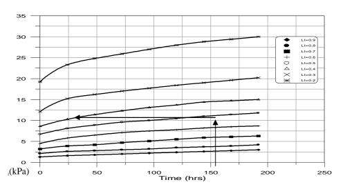
Figure (5) Variation in untrained shear strength versus time for remolded clay.
