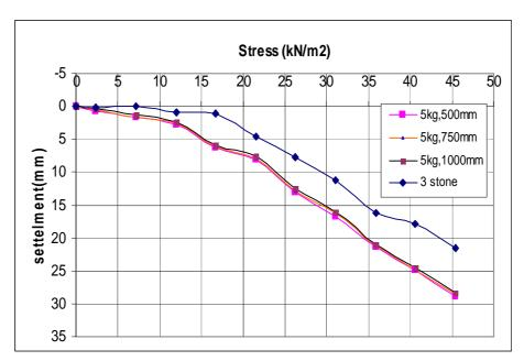
Figure (16) Stress-settlement curve for treated soil using 3 stone columns and dynamic compaction (weight 5kg , heights of drop 500,750,1000mm).
