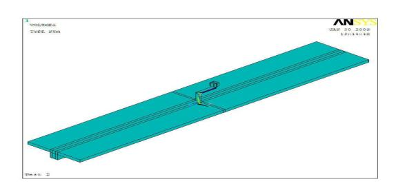
Figure (9): Floor-Single arm damper coupled system
