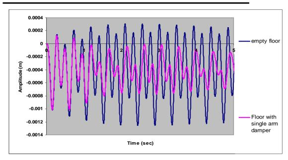
Figure (11): Transient response amplitude of the concrete floor with and without the single arm viscoelasic damper attached.
