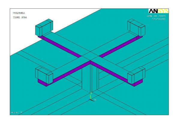
Figure (5): Four arms damper configuration
