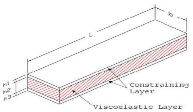
Figure (2): Constrained layers configuration [10]
