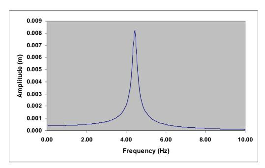
Figure (7): Fundamental frequency of floor
