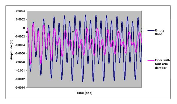
Figure (12): Transient response amplitude of the concrete floor with and without the four arms viscoelasic damper attached.
