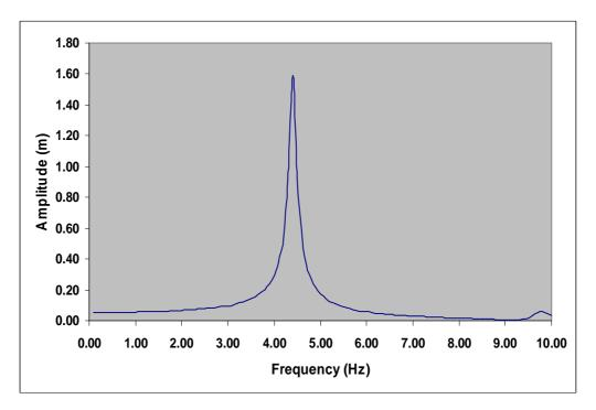
Figure (8): Fundamental frequency of damper
