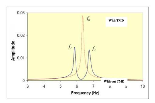
Figure (1): An example showing the effects of attaching a TMD to a primary system [10]
