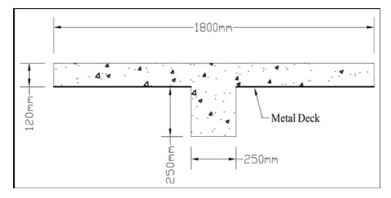
Figure (6): Concrete floor cross sectional area
