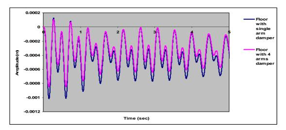
Figure (13): Comparison between transient response amplitudes of the concrete floor with the single arm or the four arms viscoelasic damper
