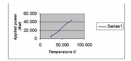
Figure (4) Temperature rise as a function of applied power on the specimen. Operation
