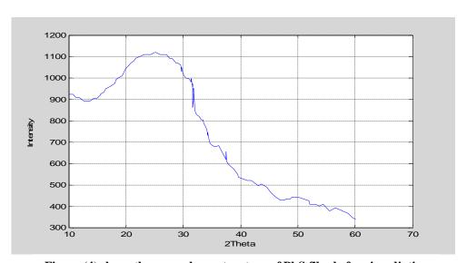
Figure (4) show the amorphous structure of PbS film before irradiation
