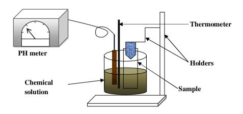
Figure (1) show the setup of deposition system
