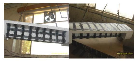
Figure (20) Mode of Failure of Strengthened Beam B690WFL (90° Strips + Long. Strips)
