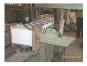
Figure (8) Clamping Torsional Arm
