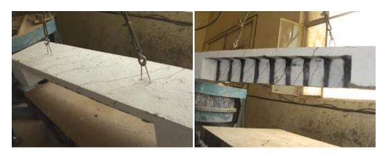
Figure (13) Mode of Failure of Strengthened Beam **B290W** (90° Strips in the Web Only)
