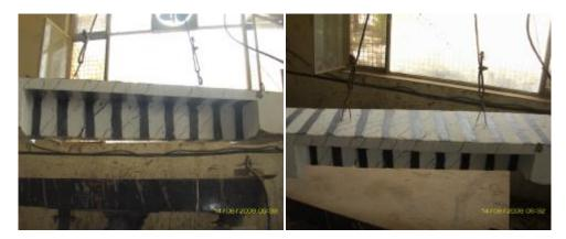
Figure (14) Mode of Failure of Strengthened Beam B390WF (90° Strips in the Web and Flange)
