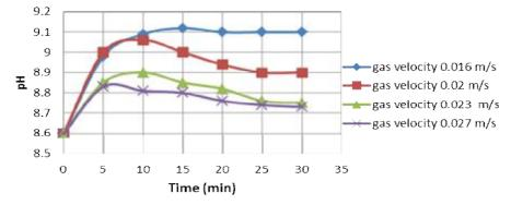
Figure(5) Effect of the gas velocity on the pH with time
