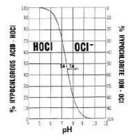
Figure(2) Ionization curve of HOCl as a function of pH [6]
