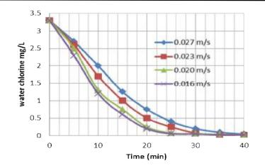
Figure( 9)Effect of the exposure time on the content of chlorine With 5 gm/L of activated carbon.
