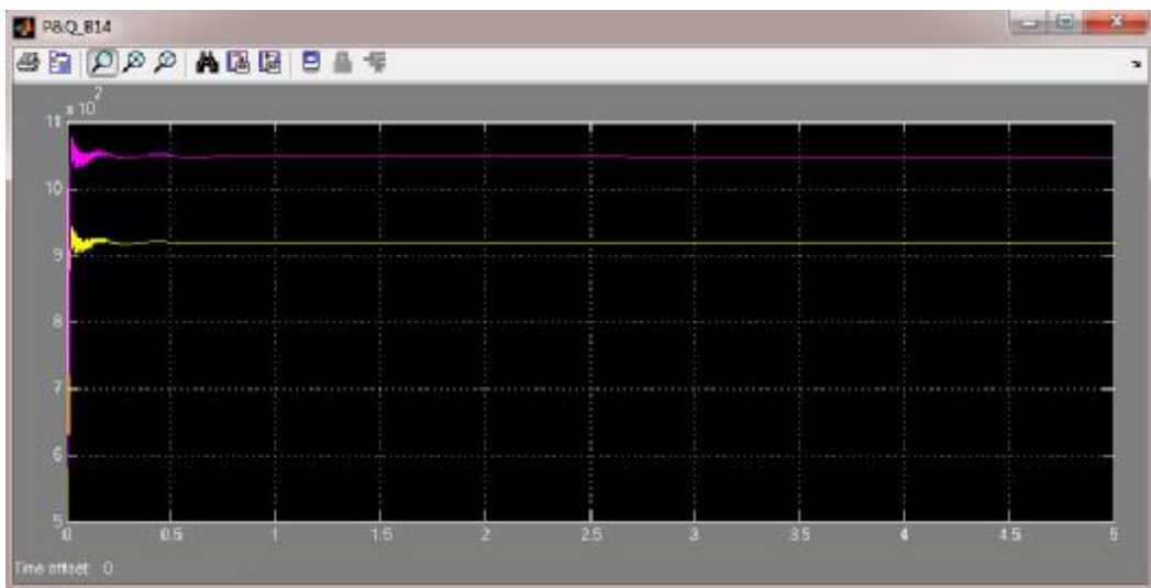
Figure (24) active and reactive power with STATCOM during maximum load with PI controller
