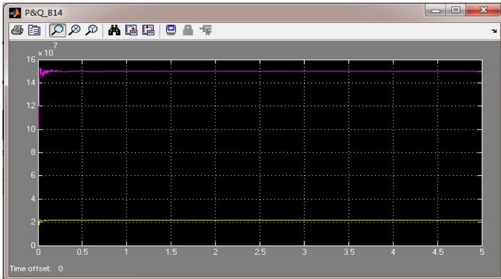
Figure (26) active and reactive power with STATCOM during minimum load with PI controller
