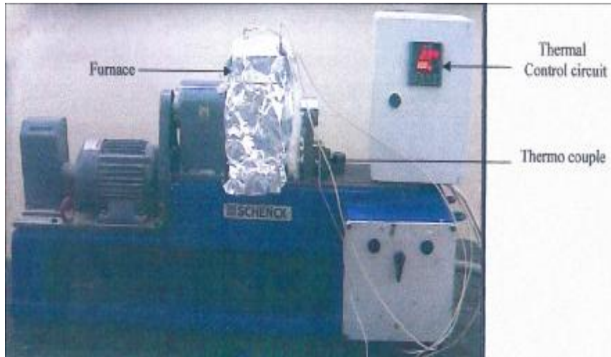
Figure (2 b) the fatigue-creep testing machine with furnace
