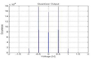
Figure (12): The output level histogram of quantizer.
