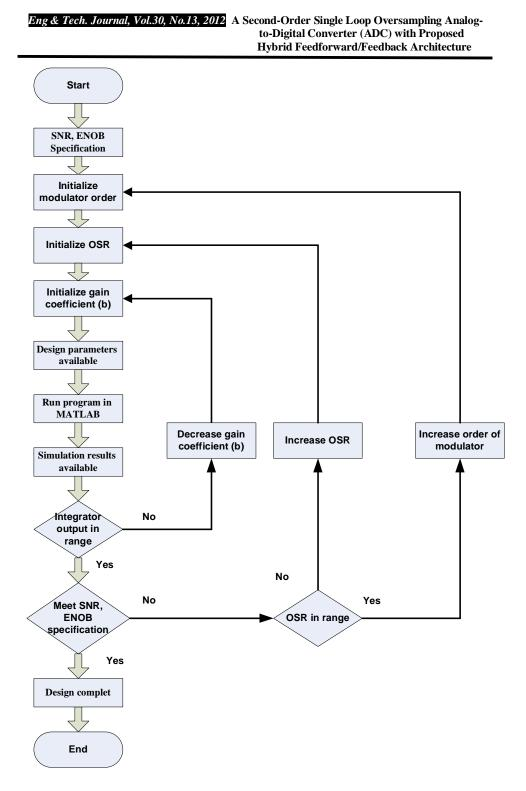
Figure (4): Flow chart of the simulation program.
