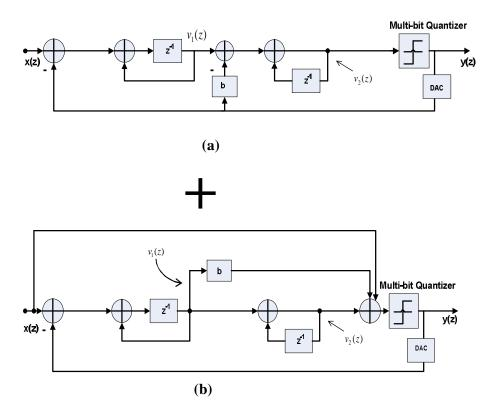
Eng & Tech. Journal, Vol.30, No.13, 2012 A Second-Order Single Loop Oversampling Analogto-Digital Converter (ADC) with Proposed Hybrid Feedforward/Feedback Architecture
