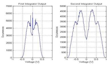
Figure (11): The output level histograms of the first and second integrators for proposed ADC.
