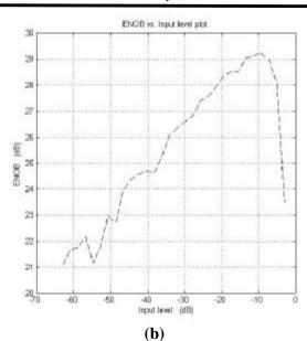
Figure(7): (a) The SNR versus the input signal power, (b) The ENOB versus the input signal power.
