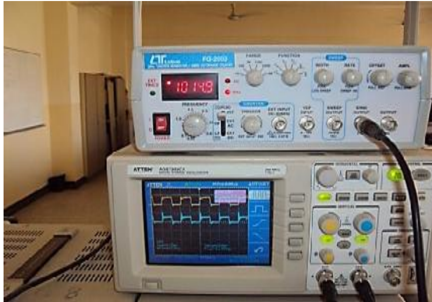
Figure (19): Input and output signal from an oscilloscope with 16-QAM.
