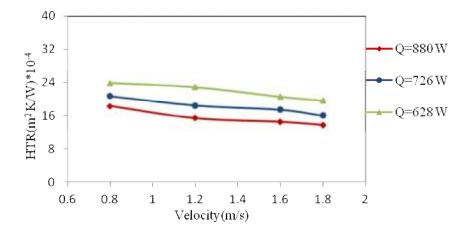
Figure (6) Variation of heat transfer resistance with velocity for treated brass with ferrous sulfate at different applied heat, at 30°C.
