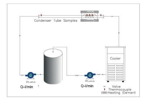
Figure (2) Thermal measurements System.
