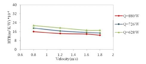
Figure (5) Variation of heat transfer resistance with velocity for untreated brass tubes at different applied heat, at 30°C.
