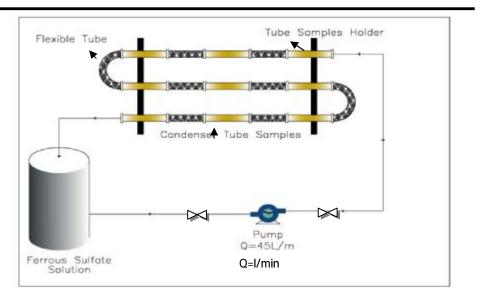
Figure (1) Ferrous sulfate treatment system.
