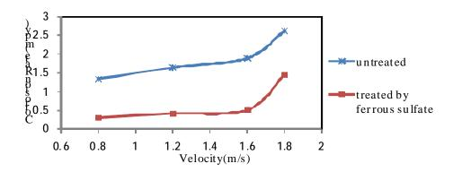
Figure (4) Variation of corrosion rate with velocity of treated and untreated brass with ferrous sulfate and filtered water(pH 7.6)respectively for 7 days, ,at 27°C.
