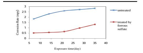
Figure (3) Variation of corrosion rate with time for treated and untreated brass with ferrous sulfate and filtered water (pH 7.6) respectively, velocity1.6 m/s , at 25°C.
