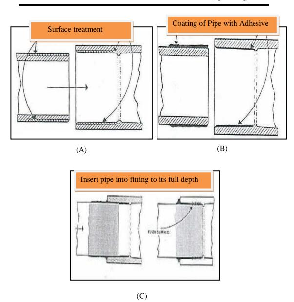
Figure (1) (A, B, C) Appearance of stages of surface Treatment for PVC pipe samples.
