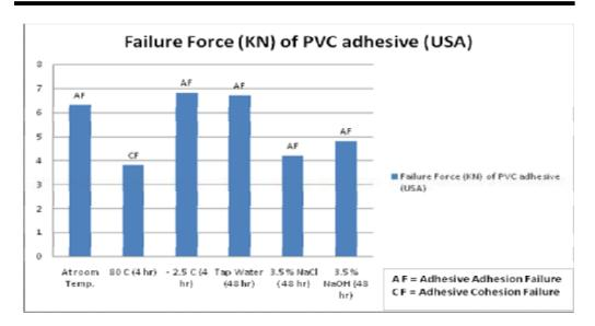
Figure (3) show results of pipe adhesion testing for PVC pipe with PVC adhesive (USA) without surface treatment, under environmental conditions.
