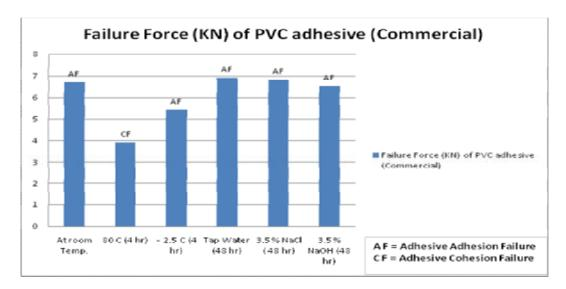
Figure (5) show results of pipe adhesion testing for PVC pipe with PVC adhesive (Commercial) without surface treatment, under environmental conditions.
