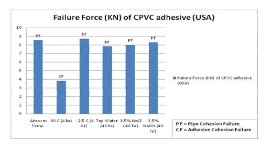
Figure (7) show results of pipe adhesion testing for PVC pipe with CPVC adhesive (USA) with surface treatment, under environmental conditions.
