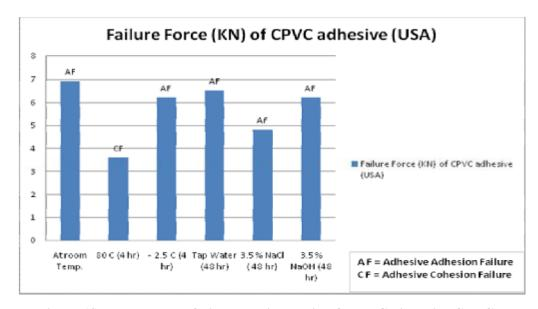
Figure (4) show results of pipe adhesion testing for PVC pipe with CPVC adhesive (USA) without surface treatment, under environmental conditions.
