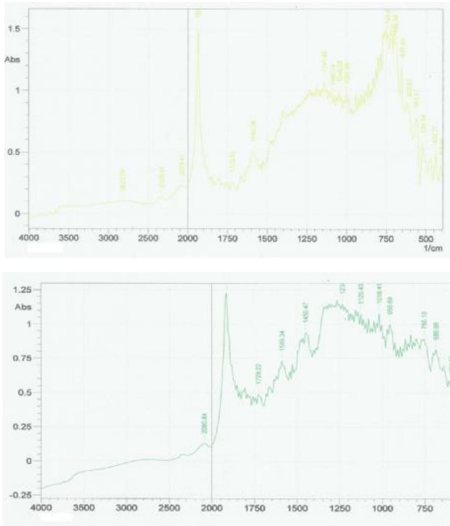
Figure (6): FTIR structure of the TiO 2 /glass thin films at different laser energy a) 800 mJ, b) 1000 mJ respectively.
