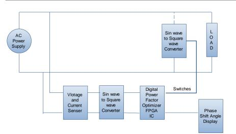
Figure (1): Digital power factor optimizer block diagram.
