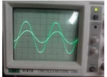
(e) phase shift between the voltage signal and current signal
