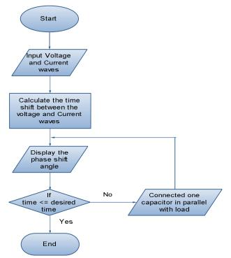
Figure (4): The flowchart of digital power factor optimizer.
