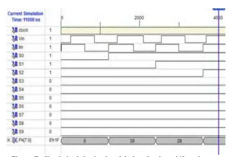
Figure (7): Simulation behavioral model when the phase shift angle greater than desired value (three capacitors are connected).
