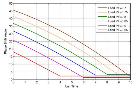
Figure (11): The relationship between the phase shift angle and the time at variable load.
