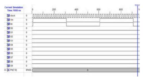
Figure (5): Simulation behavioral model when the voltage in phase with current.
