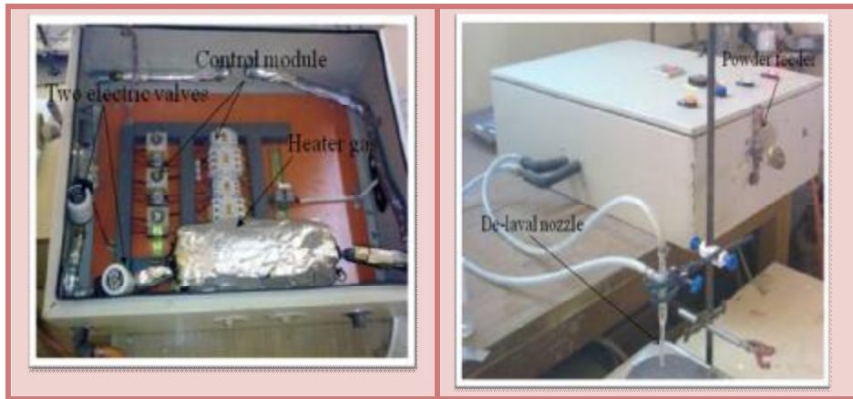
Figure.(2) Images explain the interior and external parts of the apparatus.
