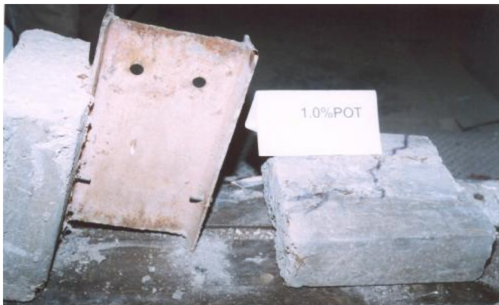
Figure (13): Photograph of Tested POT Specimen Showing the Failure mode.
