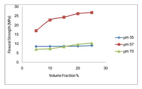
Figure (2): The flexural strength for mica filled UP composites with different filler loading.
