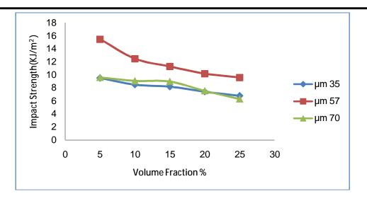
Figure (1): The impact strength for mica filled UP composites with different filler loading.
