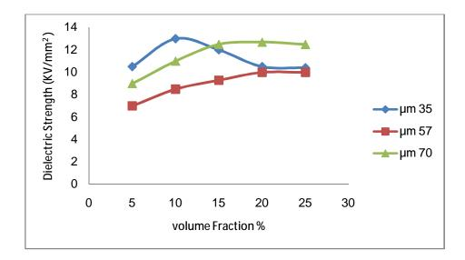
Figure(3): The dielectric strength for mica filled UP composites with different filler loading.
