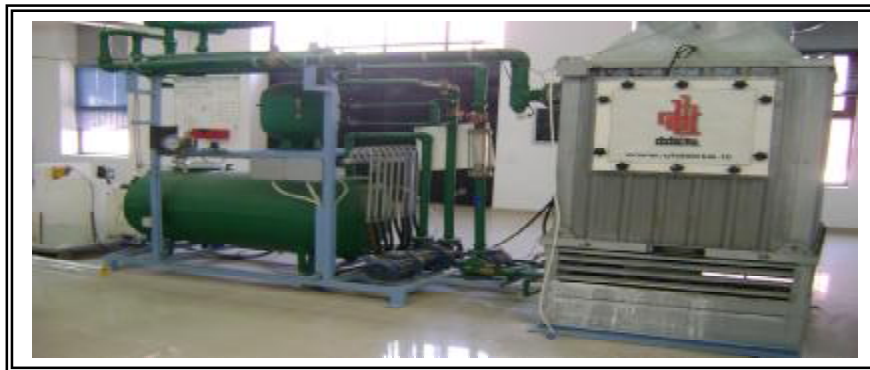
Figure (1) Condenser and cooling tower contact in steam power plant (Didacta- Italia).
