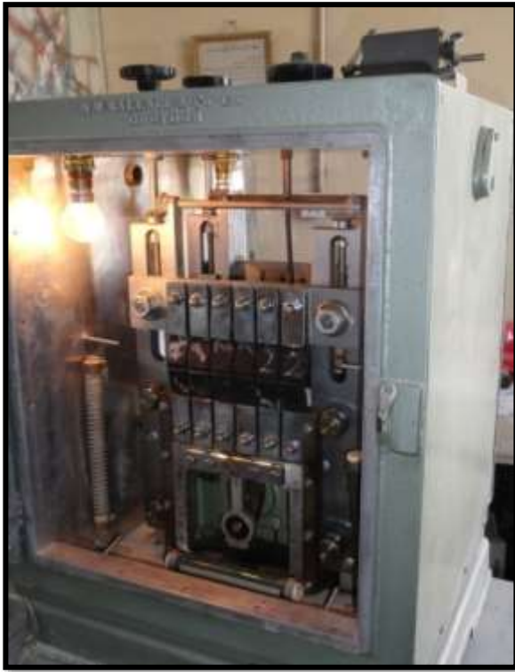
Figure (4): De Mattia Flexing Machine Test. (Made in England)
