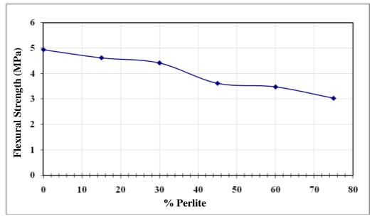
Figure (3): Relationship between the flexural strength and content of perlite as a partial replacement by volume of silica sand
