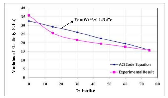
Figure (5): Relationship between the modulus of elasticity (for experimental result & ACI equation) and content of perlite as a partial replacement by volume of silica sand
