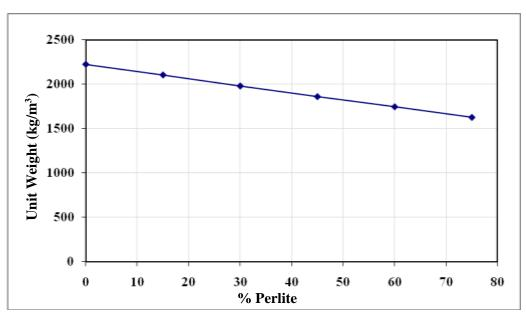
Figure (6): Relationship between the oven dry unit weight and content of perlite as a partial replacement by volume of silica sand
