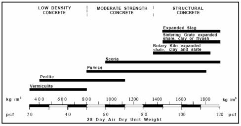
Figure (1): Approximate Unit Weight and Use Classification of Lightweight Aggregate Concrete [1].
