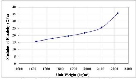
Figure (9): Relationship between the modulus of elasticity and oven dry unit weight
