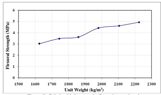
Figure (8): Relationship between the flexural strength and oven dry unit weight
