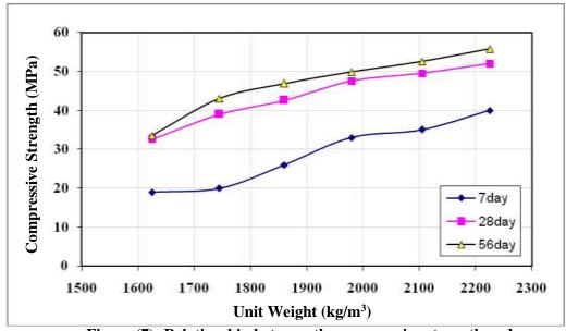
Figure (7): Relationship between the compressive strength and oven dry unit weight
