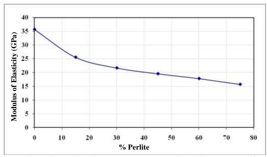
Figure (4): Relationship between the modulus of elasticity and content of perlite as a partial replacement by volume of silica sand
