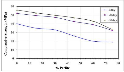
Figure (2): Relationship between the compressive strength and content of perlite as a partial replacement by volume of silica sand
