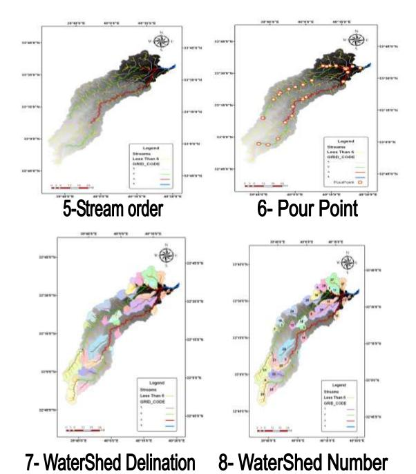
Figure (4) Stages of extracting the drainage net.
