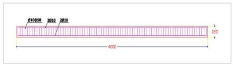
Figure (2) Geometry and reinforcement of the tested RC specimens.
