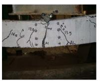
Figure (15) cracks pattern of beam (B2).
