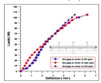
Figure (22) Load – Deflection curve for beam (B5).
