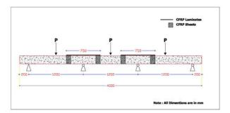
Figure (4) Schematic of specimen B2 with bonded CFRP strips
