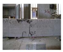
Figure (13) cracks pattern of beam (B1).
