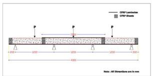
Figure (11) Schematic of specimen B9 with bonded CFRP strips.
