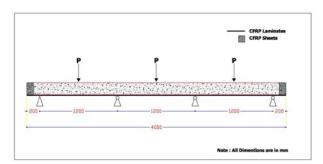
Figure (7) Schematic of specimen B5 with bonded CFRP strip.
