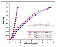
Figure (18) Load – Deflection curve for beam (B3).
