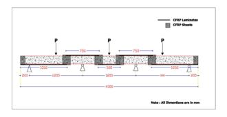
Figure (8) Schematic of specimen B6 with bonded CFRP strips.
