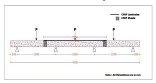
Figure (5) Schematic of specimen B3 with bonded CFRP strip.
