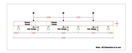
Figure (12) The locations adopted for measuring deflections and longitudinal strains
