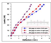
Figure (14) Load – Deflection curve for beam (B1).
