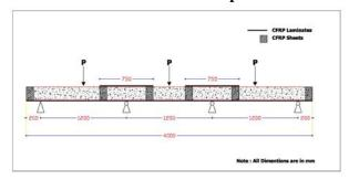
Figure (9) Schematic of specimen B7 with bonded CFRP strips.
