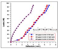
Figure (24) Load – Deflection curve for beam (B6).
