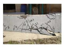
Figure (23) cracks pattern of beam (B6).
