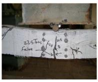
Figure (17) cracks pattern of beam (B3).
