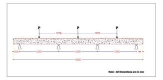
Figure (3) Schematic of specimen B1 without bonded CFRP strip.
