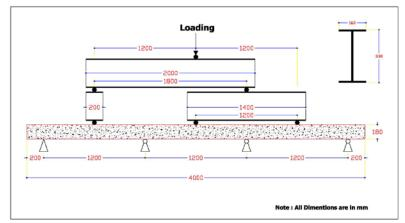
Figure (1) ) Schematic representation of tested beams.
