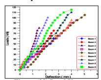
Figure (33) Load Versus Deflection at center of middle span for the beams.
