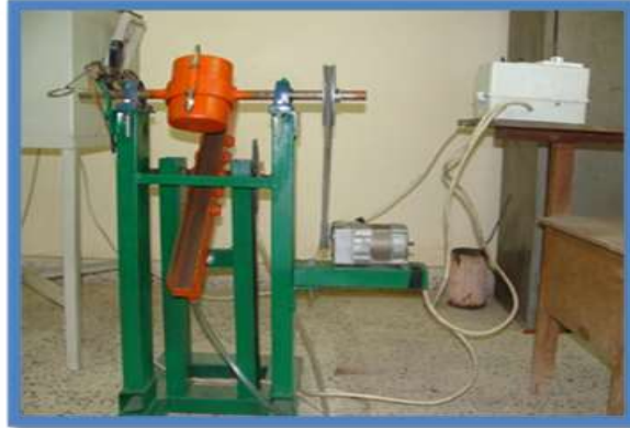
Figure (1) Photograph of the Slope Plate Casting unit Used in this work.
