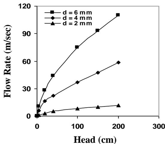
**Figure (2) Calibration curves for the pinhole test using aluminum cylinder sample**
