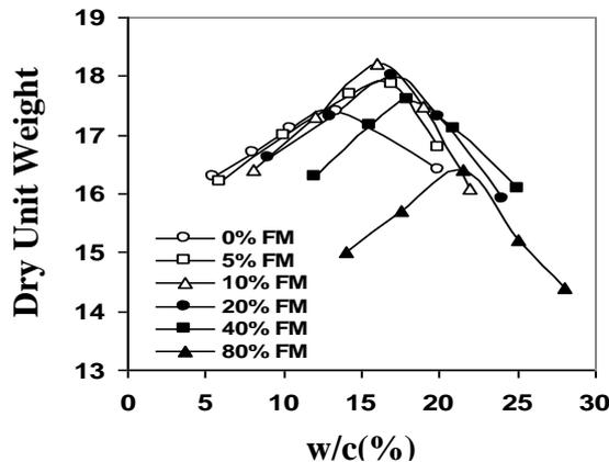
**Figure(3) Compaction curves of natural and treated soil with different percentages of fine materials.**
