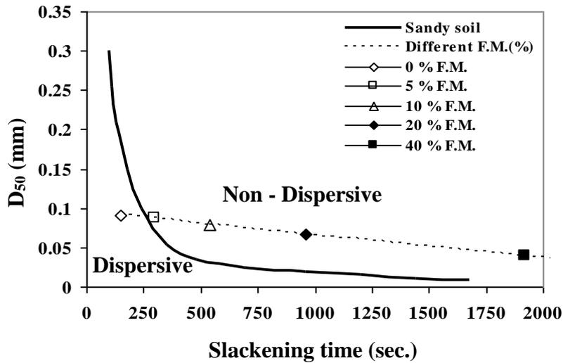
**Figure (5) Diagram developed for evaluation of physical dispersivity based on slackening time.**
