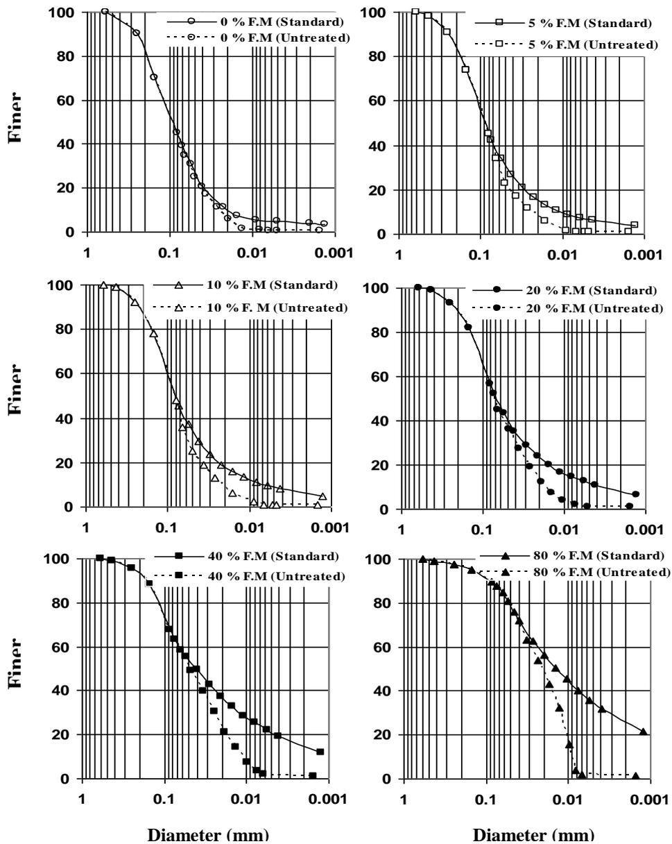
Figure (4) Grain size distribution curves for double hydrometer test with different percents of fine materials.
