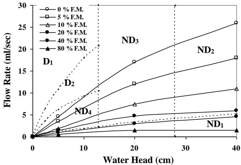
Figure (7) Classification curves of soil by pinhole test.
