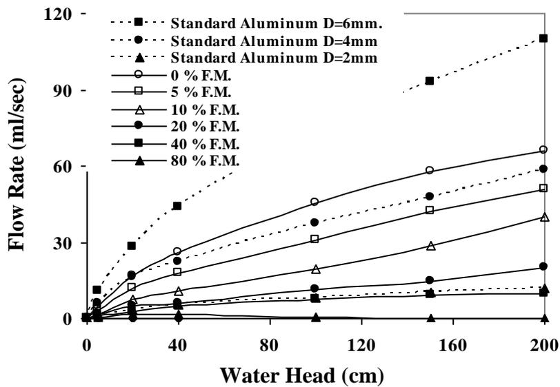
**Figure (6) Variation of flow rate and hole size with water head and fine materials additions .**
