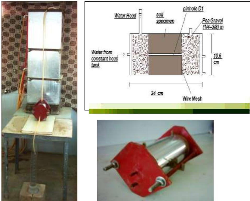
**Figure (1) Testing device with all apparatuses.**
