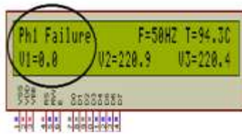
(a) Ph1 failure
