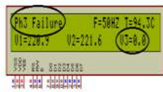
(c) Ph3 failure
