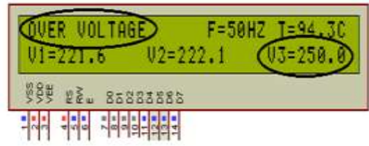
(b) Ph3 Over voltage.
