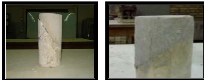
(a) Slant surface failure (b) Material failure Figure (4) Failure of the composite slant sections of the research.
