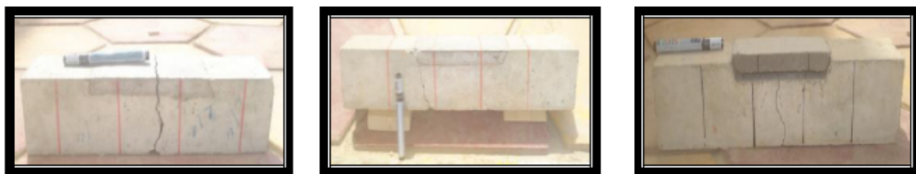
Figure (6) Failure modes of composite section beam, (a) the failure at the centre, (b) the failure at edge of the notch section, and (c) the failure as delamination notch section.
